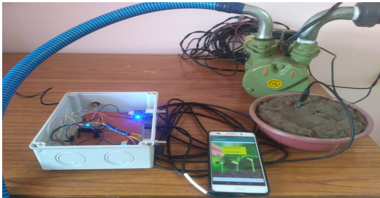
Figure 3: Prototype of Android mobile based smart water- saving Irrigation system.
